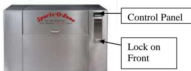
Underneath the control panel inside the door is a small "black" toggle switch. Slide the toggle switch forward to put the computer board into program mode. This option allows the owner of the machine to reset the date and time on the machine, the lock out security code, or to change the dollar amount he or she would want to charge on the vending models. COUPONS DO NOT HAVE A VALUE. THIS PROGRAM CHANGE ONLY AFFECTS DOLLARS ACCEPTED OR CREDIT CARD CHARGE.
